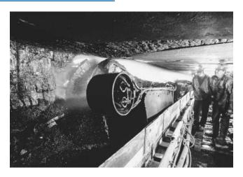
A longwall shearer cuts swatches of coal 750 feet long and 28 inches thick, 800 feet underground at Consolidation Coal Company's Blacksville #2 mine. (Corbis-Bettmann)
