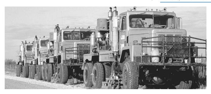
This is a team of trucks that create and record seismic vibrations, in an attempt to detect the presence of oil. (Corbis Corporation)
