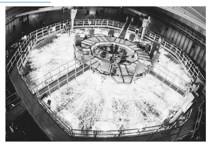
Particle beam fusion accelerator II (PBFA-II) was designed to deliver at least 100 trillion watts of power and was the first machine with the potential to ingnite a controlled laboratory fusion reaction. (U.S. Department of Energy)
