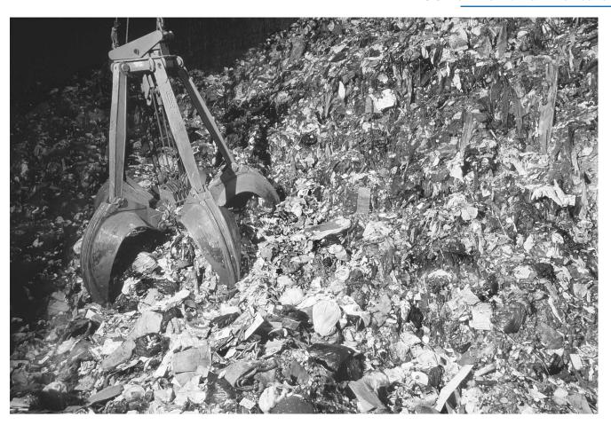
The Bridgeport RESCO power plant mixes garbage to facilitate the drying process, which improves the efficiency of energy generation by incineration. (Corbis Corporation)
