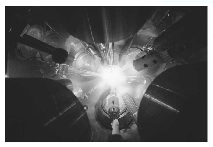
Lasers are focused on a small pellet of fuel. This is an attempt to create a nuclear fusion reaction for the purpose of producing energy. (Corbis-Bettmann)
