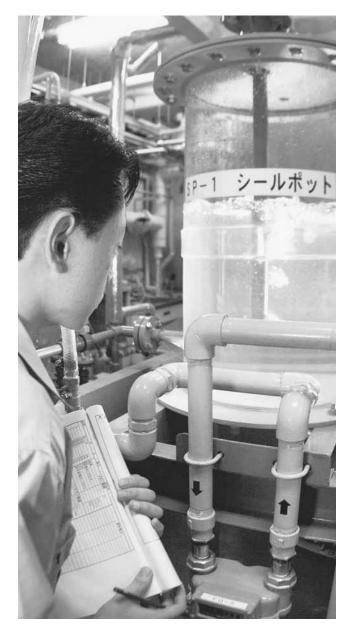
A researcher checks a sealed poy of methane in Kajima Corp.'s newly developed system designed to break down organic waste. (Corbis-Bettmann)
